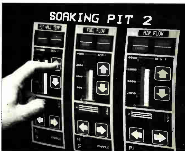
MOVING FINGER. Used mostly for military and industrial-process applications, touch screens are poised to find a wider market.
