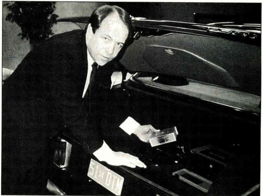
JUKEBOX IN TRUNK. Sony's CDX-A10 DiscJockey has magazine and changer mechanism.
