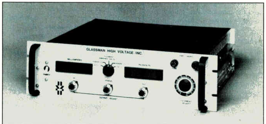
Rf power supplies, such as Glassman's high-voltage products, are inherently safer than 60-Hz supplies because less energy is stored in the capacitors used for filtering. Applications include flying-spot scanners, X-ray sources, and flocking systems.
