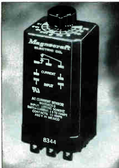
A silicon controlled rectifier and bridge arrangement are used in Magnecraft's ac sensing relay to avoid loading the circuit being monitored. Its output is a single-pole double-throw relay rated at 10 A.
