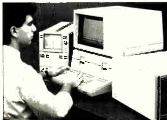
MENU. Users create waveforms on HP's 8770S generator by picking elements like ramps or random noise from a menu.
