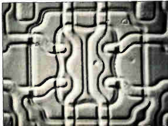
FEATURED IN 3-D. The IVS system features an image-shearing function that gives 3-d effects to irregularities.
