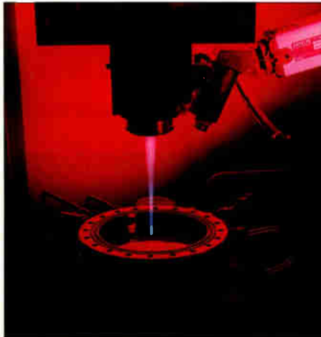
THIN LAYERS. XMR's doping system uses an XeCl gas laser to form controllable diffusion junctions in substrates 500 to 1,200 Å deep.
