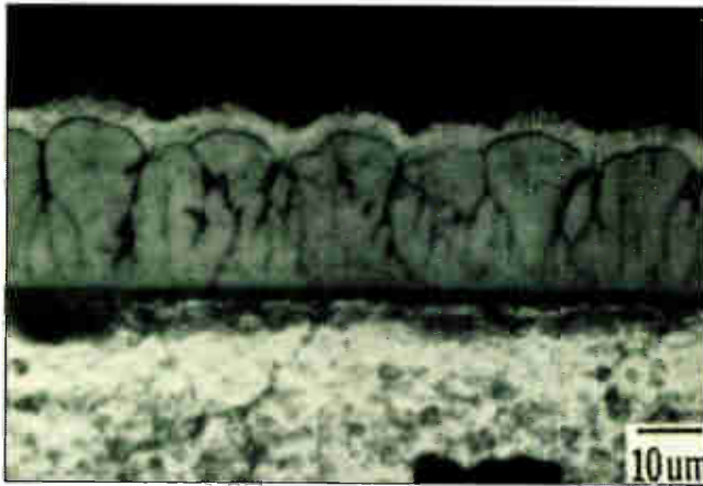
CLEANER. Laser-jet-plated gold spots, top, compared to depositions without use of laser power. In both cross-sections, top layer is nickel, then come gold, nickel plating, and beryllium copper substrate.
