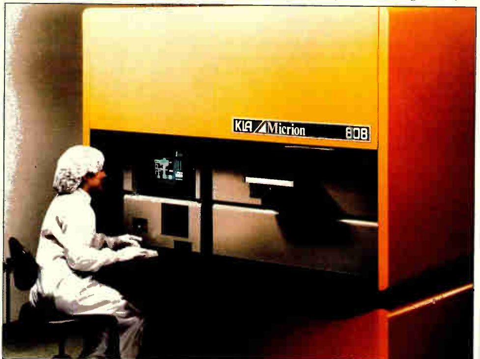
1. FIXER. The KLA/Micrion 808 uses an ion beam to mill out defects in optical and X-ray masks.
