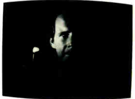
The CCD registers detail with as little as 3 lux (0.3 footcandle) illumination.
