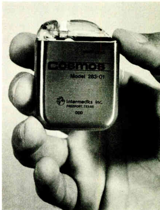
Pacer. Built around a custom 8-bit microcomputer, Intermedics' Cosmos pacemaker can store diagnostic data for the physician that has generally not been available.
