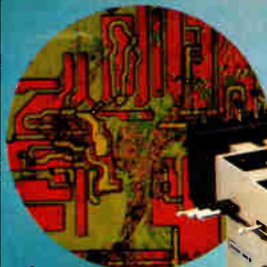
"Contamination defects at 300X found during wafer inspection"
