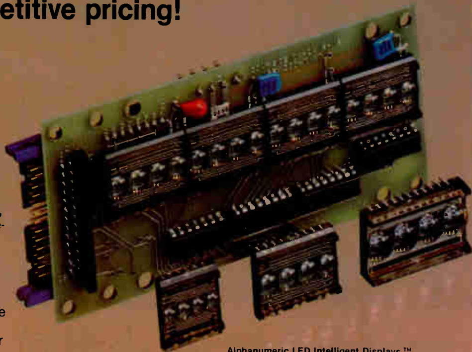
Alphanumeric LED Intelligent Displays™ 4 and 8 character LED Display modules with 16, 17 or 22 segment font and on board CMOS integrated circuit. The CMOS chip provides segment decoding, drivers, multiplexing and memory for easy interfacing to most microprocessors. Also available mounted on boards in 16 and 32 character assemblies.
