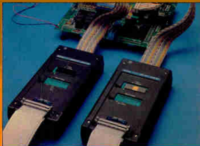
Multi-emulation in a 2-microprocessor system.
