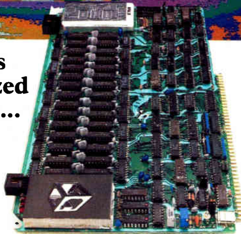
In 17 msec. the image above was viewed by a camera, stored in memory, retrieved, and displayed in pseudo-color. This VG-120 board made it possible.
