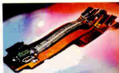
The missile's autopilot and battery circuits of PYRALUX consist of two 4-layer flat cable assemblies containing power, signal, and shielded digital circuits.
