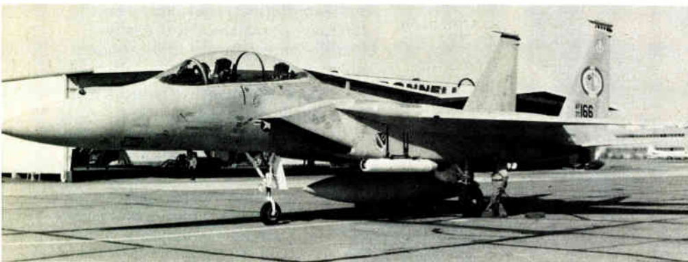
Equipped. This is the F-15 fighter aircraft now flying at Edwards Air Force Base in California and equipped with a laser target-tracking pod suspended beneath the port intake.
