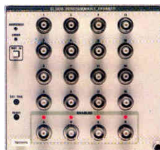
SI 5010 Programmable Scanner Interface • 350 MHz Coaxial Switching • Software Reconfigurable as: 16 Channel to 1 dual 8 Channel to 1 quad 4 Channel to 1 • Buffered Mode for Controller Unattended Operation • Real Time Clock • Triggered Events
