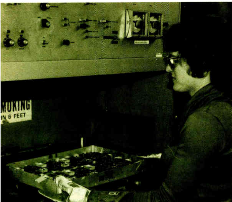
2. Vapor-phase soldering. One of the keys to successful mounting of leadless chip-carriers and other leadless components on standard pc-board surfaces is vapor-phase soldering. In this operation, all solder joints are fused simultaneously in an oxygen-free environment.
