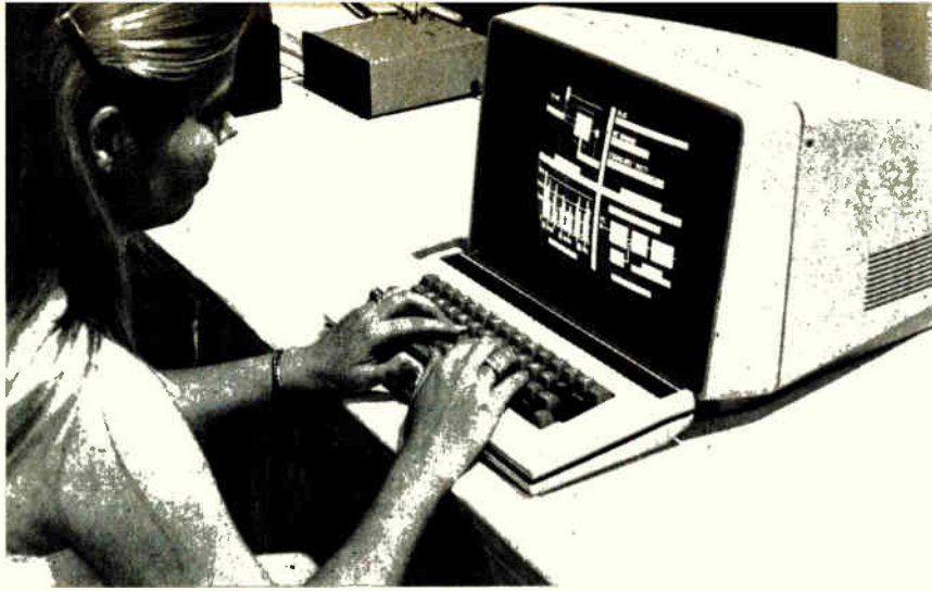
Capable. Twelve-inch-diagonal screen of Integrated Terminals' eight-color model 801 is set up to demonstrate several of the types of graphics displays it can present.
