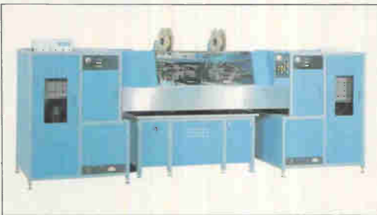
Auto load consists of a single cabinet which contains both input and output sections. It is mounted to the left of a single head VCD and one on each side of a dual head machine. Unpopulated boards are stacked in the input section. They are automatically fed to the insertion machine, and populated boards are returned to an output magazine. The unit is controlled by a dedicated microprocessor and requires only in position and transfer complete signals from the VCD.
