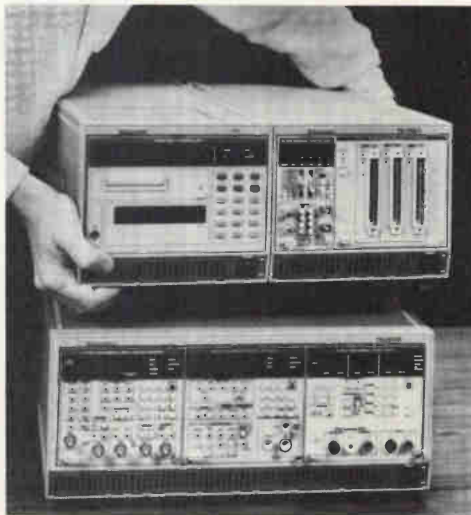
1. System building. Combining the modular design approach of the TM 500 with the IEEE-488-1978 interface standard resulted in the TM 5000 series shown above. The controller, top left, enhances IEEE-488 operation and serves both the novice operator and the advanced programmer.
