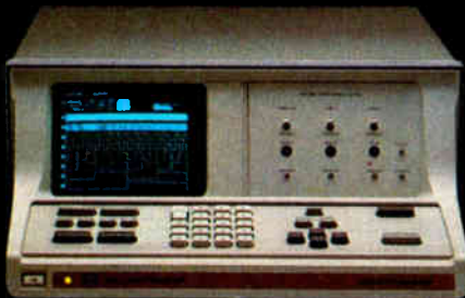
Hewlett-Packard 1615A A very good logic analyzer
