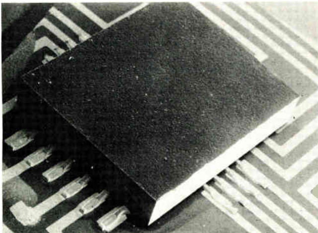
5. Face-to-face. Tape-automated bonding may be applied to hybrids in two ways. In face-up TAB (right), the chip's back is epoxy-bonded to the ceramic substrate. In face-down TAB (left), leaded chips are bonded to the ceramic face down and covered with a silicone coat.
