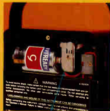
Doubly-fused protection network now conveniently located in the directly accessible battery-and-fuse compartment
