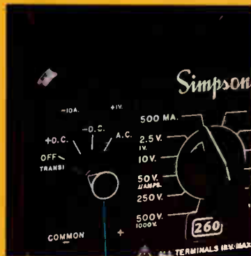
Off/Transit position of function switch shunts the meter movement and opens internal connections to the common and "+" jacks
