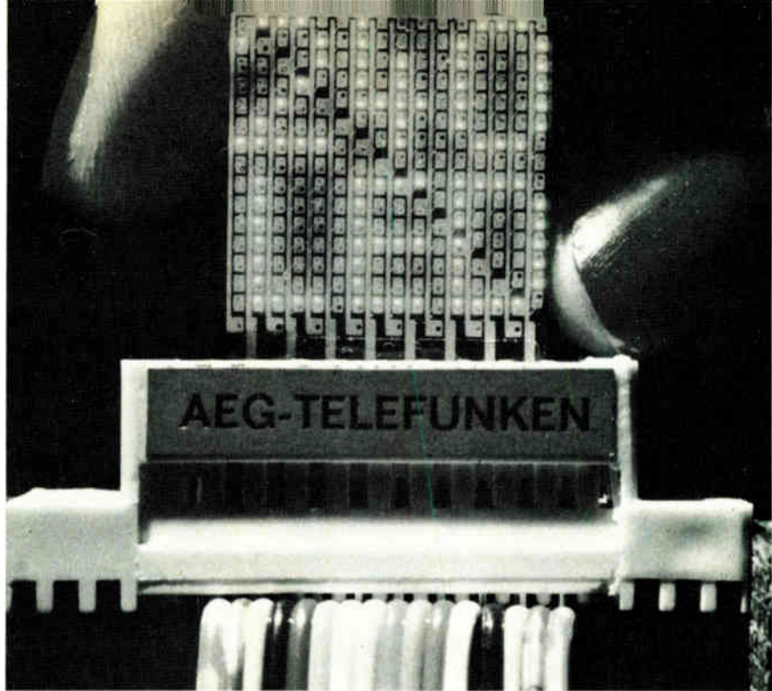
Compression. Only 16 control lines (instead of the usual 31) can drive this 240-element LED array, thanks to a new data-compression technique in Telefunken driver integrated circuit.
