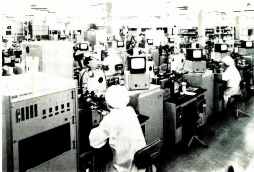
4. Machine control. Fully automated wire-bonding machines went into operation at Nippon Electric as early as 1975 to make plastic-encapsulated integrated circuits.
