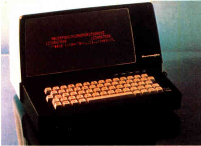
10. Terminal display. The bulky cathode-ray tube is facing competition from dc gas-discharge display technology in some applications, such as in this data terminal from Burroughs. The firm uses its own Self Scan II panel, which displays 12 lines of 40 characters each.
