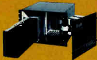
Hard disk drive at lower left can be interchanged just by sliding out and disconnecting plug. Seven free card slots are available. Z-2H includes printer interface card.
