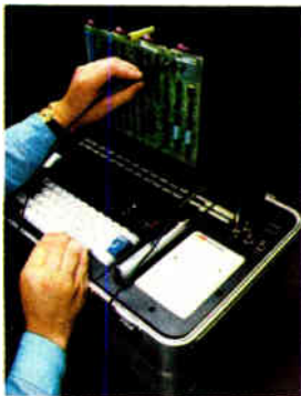
GenRad's functional field tester lets you diagnose and repair bad boards in the field, reducing spare board inventory that can tie-up 5 to 10% of your gross sales.
