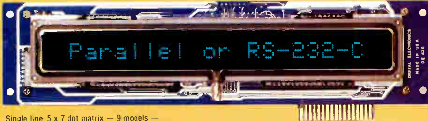
Single line 5 x 7 dot matrix — 9 models — 10, 16, 20, 32, 40 character line lengths
