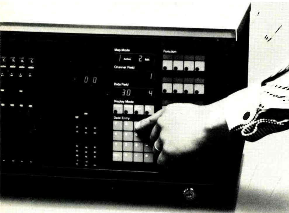
Flexible. DCX 840's network control panel allows user to reconfigure switchable data network as needed. Systems built with DCX series multiplexers can handle up to 4,000 lines.
