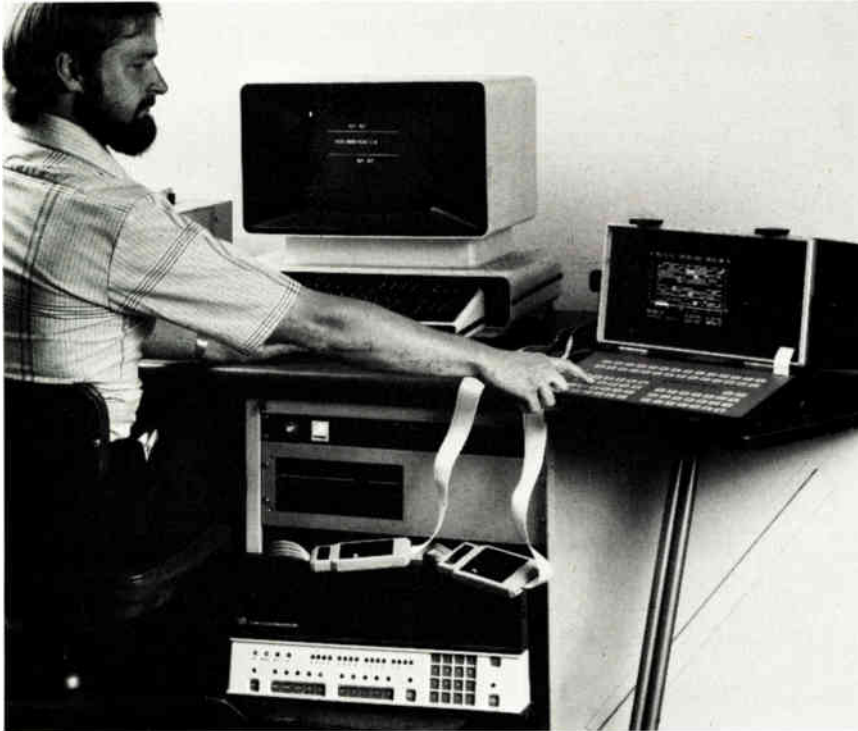
Multipurpose. Paratronics' new analyzer (right) can perform several functions, thanks to a plug-in cards holding front-end electronics and a program read-only memory.
