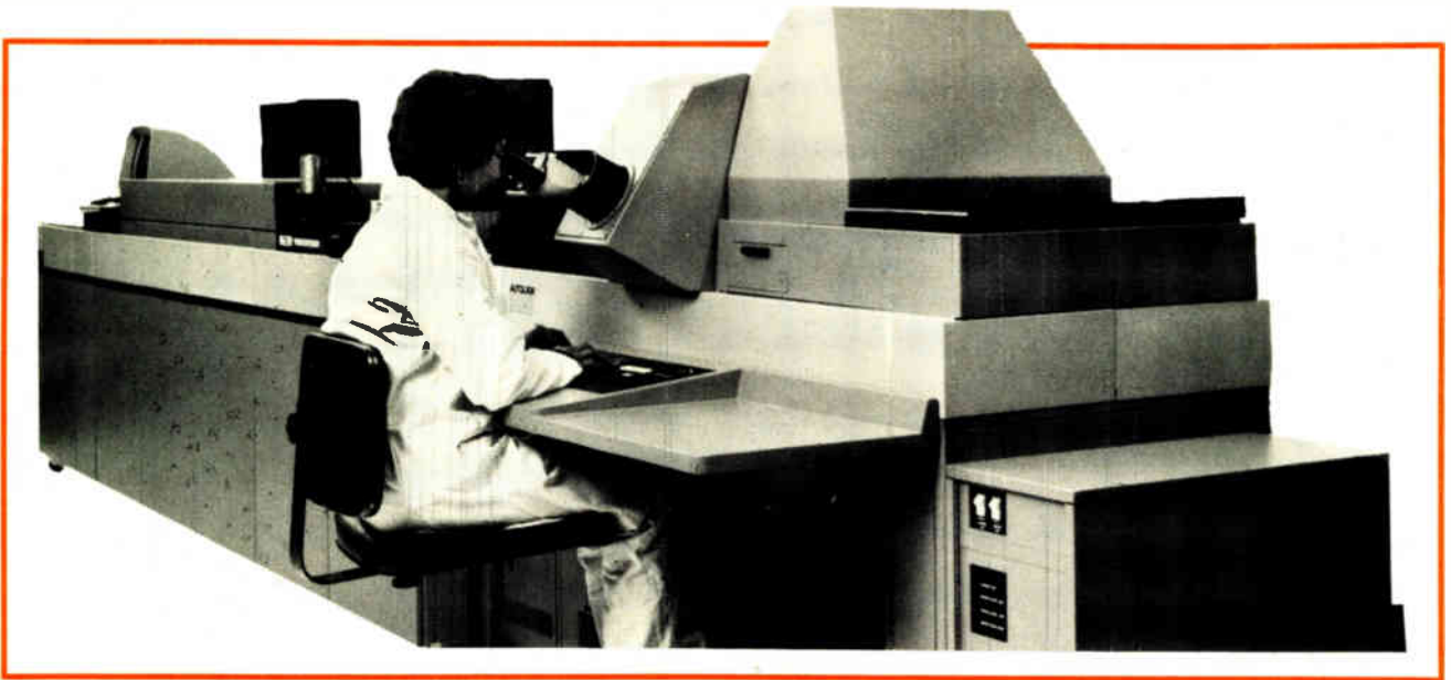
2. In line. A strong competitor to the Micralign is Cobilt's CA 3000, shown interfaced with an automatic in-line wafer-processing system. The CA 3000 features automatic mask-to-wafer alignment and can accommodate up to 92% of a 5-inch wafer.
