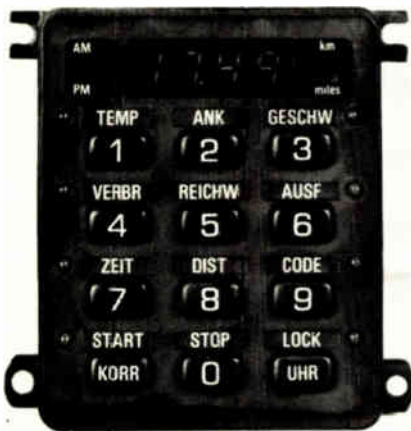
On the alert. Keyboard and display unit contains eight LEDs, to supply warnings (red), as well as information (green).
