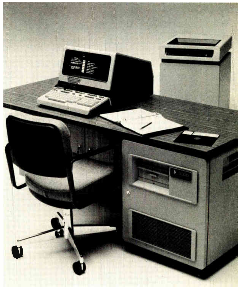
7. Versatile. The three-chip central processing unit used in the HP-300 can also be used in the HP 3000 series 33 processor shown here. Changing the voltage on the mode pin of the register, address, skip, and special chip (RASS) alters its operation.
