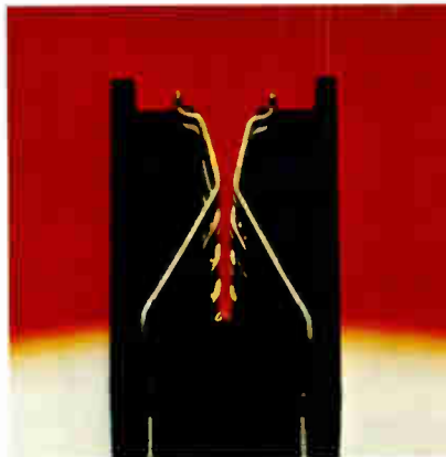
Cross Section of H4 Series Edgeboard Connector
