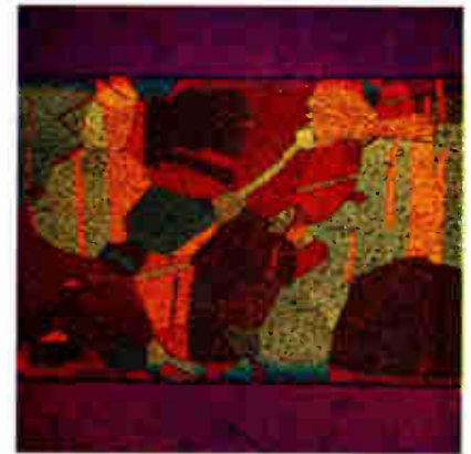
Cross section of a 3-layer pressure-bonded composite metal.
