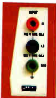
8921A's Isolated Banana Jack Input.
