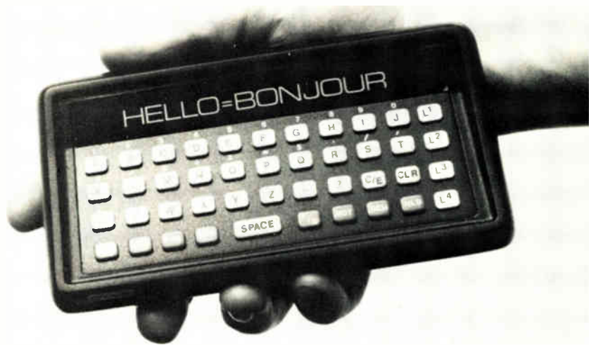
Interpreter. Craig Corp.'s electronic language translator sports 43-key, dual-function keyboard and 16-character fluorescent display. Language modules plug in from below.
