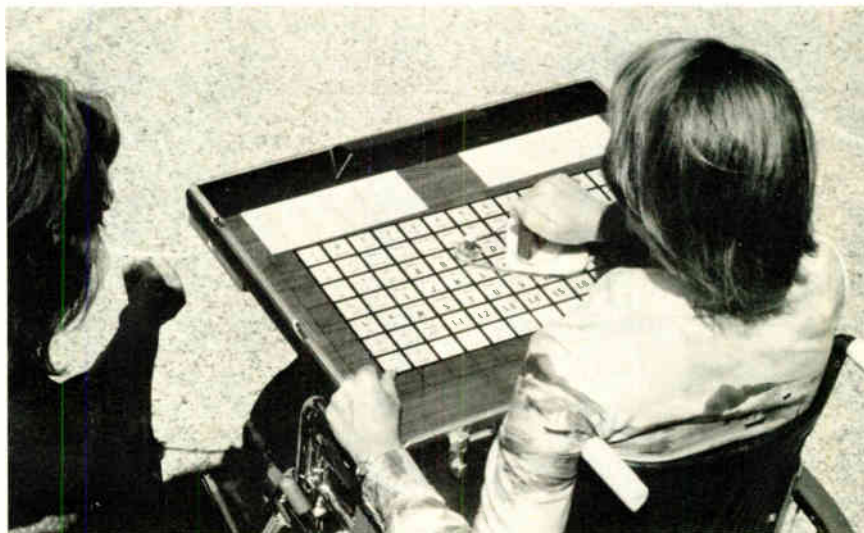
Composer. Messages, composed on Autocom by pushing magnetized pointer over letters, words, and phrases, are read on LED display housed in black rectangle at board's far edge.
