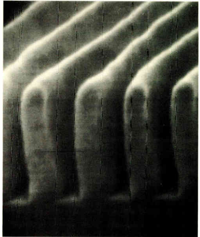
2. SEM. This scanning-electron micrograph shows a grating with 1,600-angstrom line width in PMMA photoresist that has been exposed to a copper X-ray source. (Courtesy, P. X. Flanders, Lincoln Laboratories, Massachusetts Institute of Technology.)
