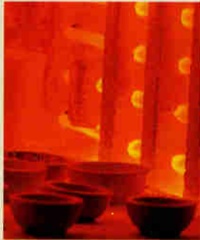
Fire assay helps Texas Instruments metallurgists determine precious metal purity, fundamental to achieving high reliability.
