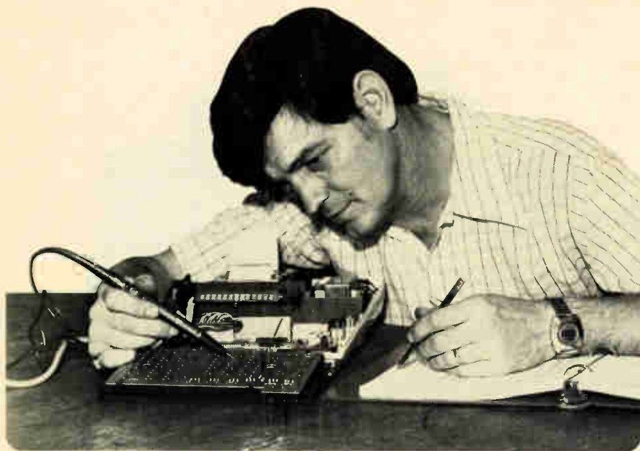
While Toshiba calculator dealers find the 545A Logic Probe a valuable service tool, a number of major customers do too. Here a technician for an oil company business machine maintenance department checks a Toshiba calculator's main circuit board for pulse activity.
