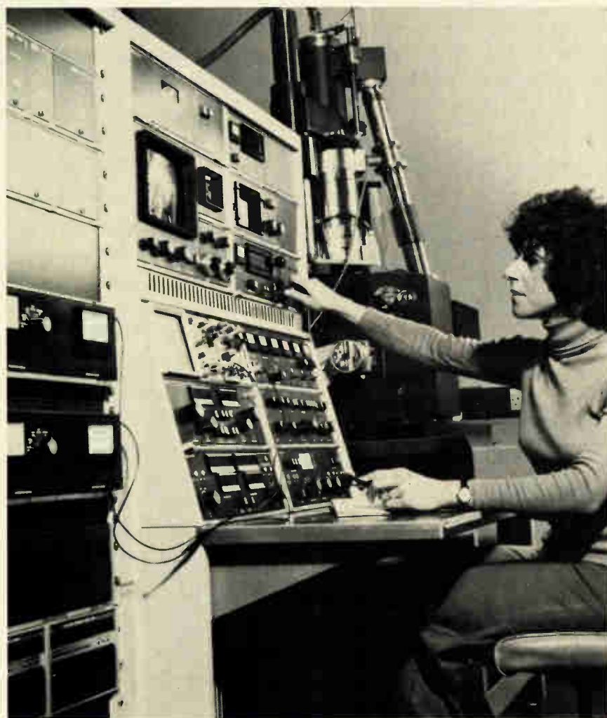
Getting it together. Electron-beam mask-making equipment is tested at the Philips Research Laboratories. Equipment would play an important role in VLSI effort.
