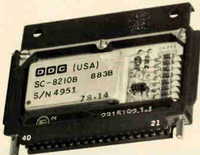
3. SEM. Many of the Navy's standard electronic modules (SEMs) consist of small thick-film substrates mounted to either ceramic or epoxy-glass motherboards. ILC Data Device Corporation uses the latter construction method in the SEM shown above.
