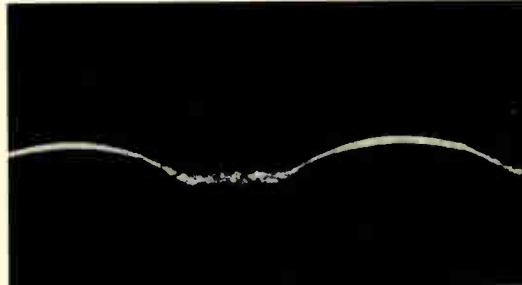
Measuring a thick-film conductor print in the wet state means no waste of substrates.
