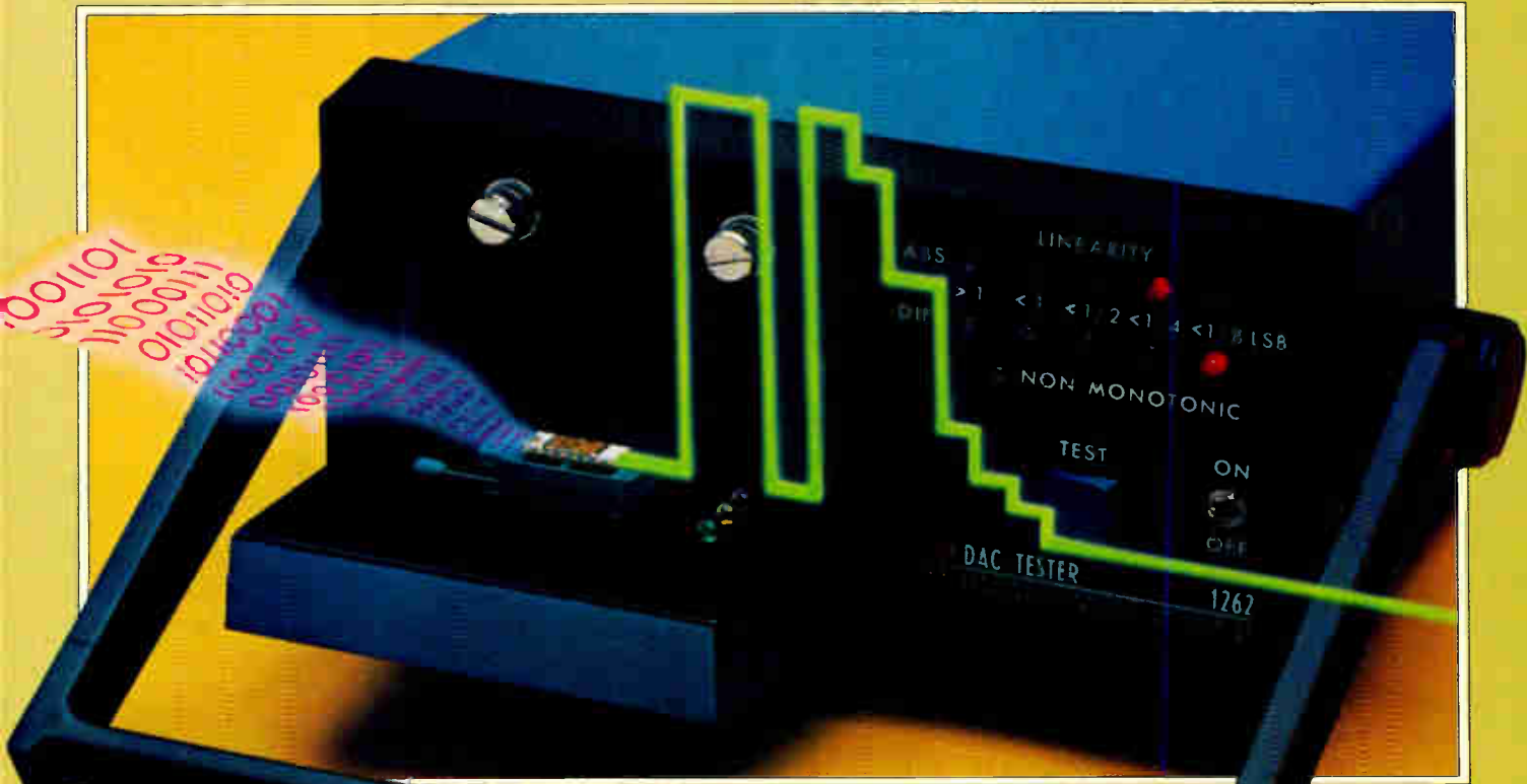
Model 1262 accurately reads wide variety of DACs for linearity, monotonicity. Price: $2960.
