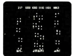
Map Mode. Each digital word can be translated into a singularly positioned dot in this graphic representation of recorded data. Especially useful for spotting illogical or illegal memory addresses.
