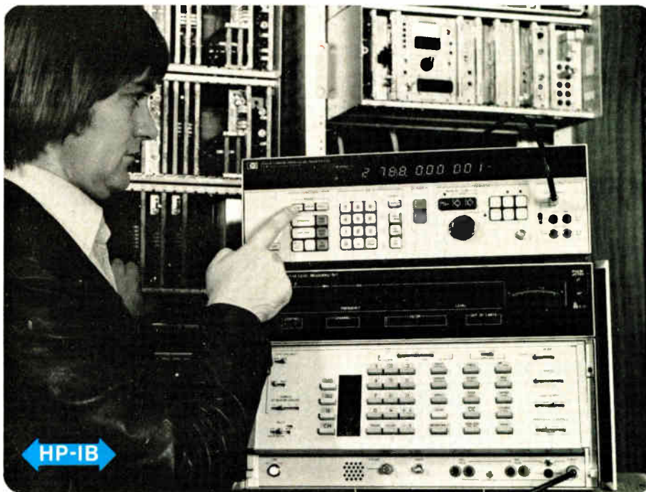
New microprocessor-based frequency synthesizer is used in applications wherever a high resolution, precision amplitude test signal is needed.
