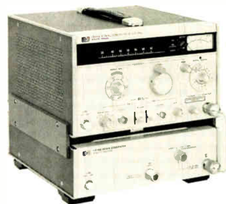
New HF down converter now covers test applications in the 10 kHz to 11 MHz band.
