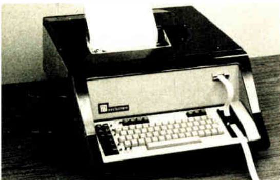
Linguist. Desk-top teleprinter, the model BT-3502, costs around $4,000, relies on PROMs to switch between alphabets.
