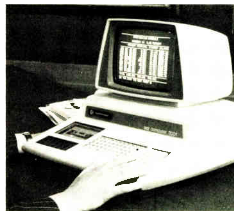
2001. $495 computer enters programs supplied by Commodore or user into cassette player built in at left of keyboard.
