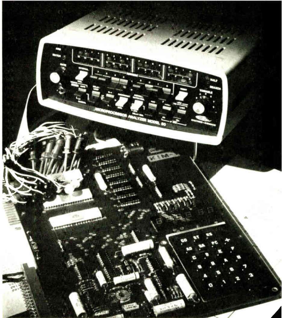
8. Generalized. Users can adapt Systron-Donner's model 50 microprocessor analyzer to handle almost any microprocessor type by changing a printed-circuit board and the test cable. A single-clip test probe can be used instead of the grabber-hooks shown.
