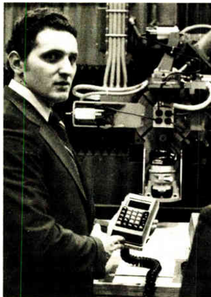
Control. Ken Susnjara holds calculator-like programmer in front of his microprocessor-controlled five-axis machining tool.
