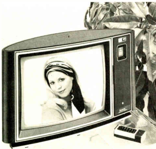
8. New tube. Zenith's Ellipse II 19-inch receiver (left) features the new Able picture tube. With its tripotential, extended-field-lens, in-line gun, the 100° deflection tube at the right below is 2½-in. shorter than present delta-gun, 90°-deflection, 19-in. models at the left.
