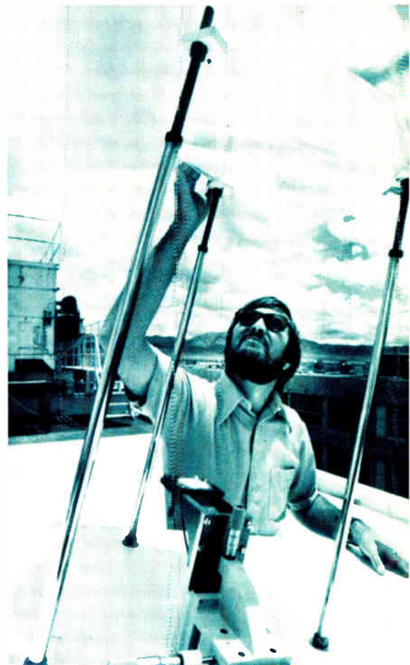
Bright outlook. Sandia Labs' approach to solar energy uses a Fresnel lens to concentrate the sun's rays on a cell. Technique is called a concentrator subsystem.
