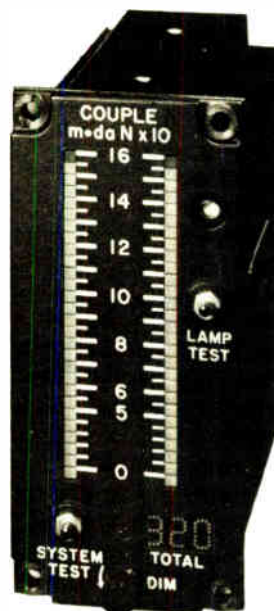
1. Glowing column. Incandescent lamps feeding light through optical fibers form a bar-graph display in this meter from Canadian Marconi. Its rugged package and bright display are designed to withstand the environment of aircraft cockpits.
