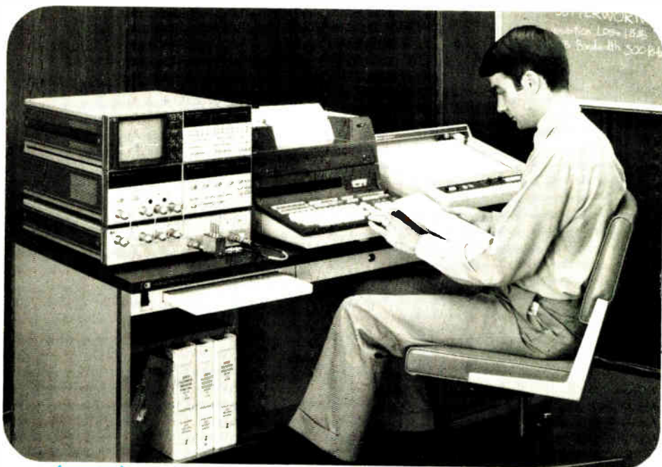
Model 8507A Automatic Network Analyzer, 500 kHz—1.3 GHz, dramatically reduces the time and cost of executing complicated tests.
