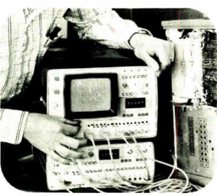
In the MAP mode, you can examine the unique "fingerprint" of every logic system.
