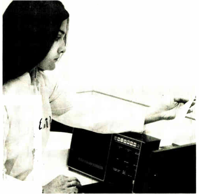
1. Test station. Blood analyzer is arranged for fast, accurate measurements. Hard-copy printout provides permanent record.
