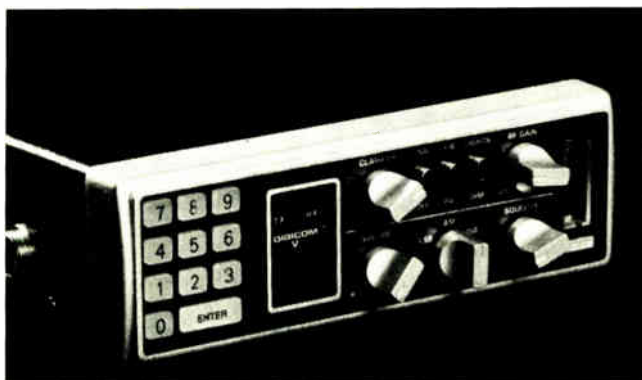
6. Selecting channels with push-button ease. SBE's phase-locked-loop synthesizer accepts keyboard inputs at a random and asynchronous rate, where all inputs are neglected except for the last two digits punched in before the enter button is pressed.
