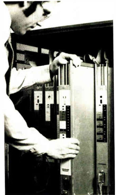
Easy fit. Elements of processor-based model 1084 programable controller from Modicon can be plugged into the unit.
