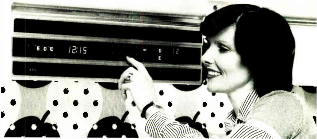
Hausfrau's friend. Programs for cooking, baking and frying are selected via overhead push buttons in AEG-Telefunken's electric range. Microprocessor-based electronic unit stores 120 cooking programs for different dishes—anything from doughnuts to ducklings.
