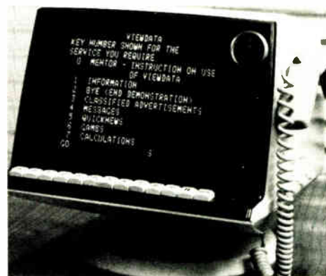
Screen test. British post office's Viewdata system links television terminals with telephone lines to display data for subscribers.
