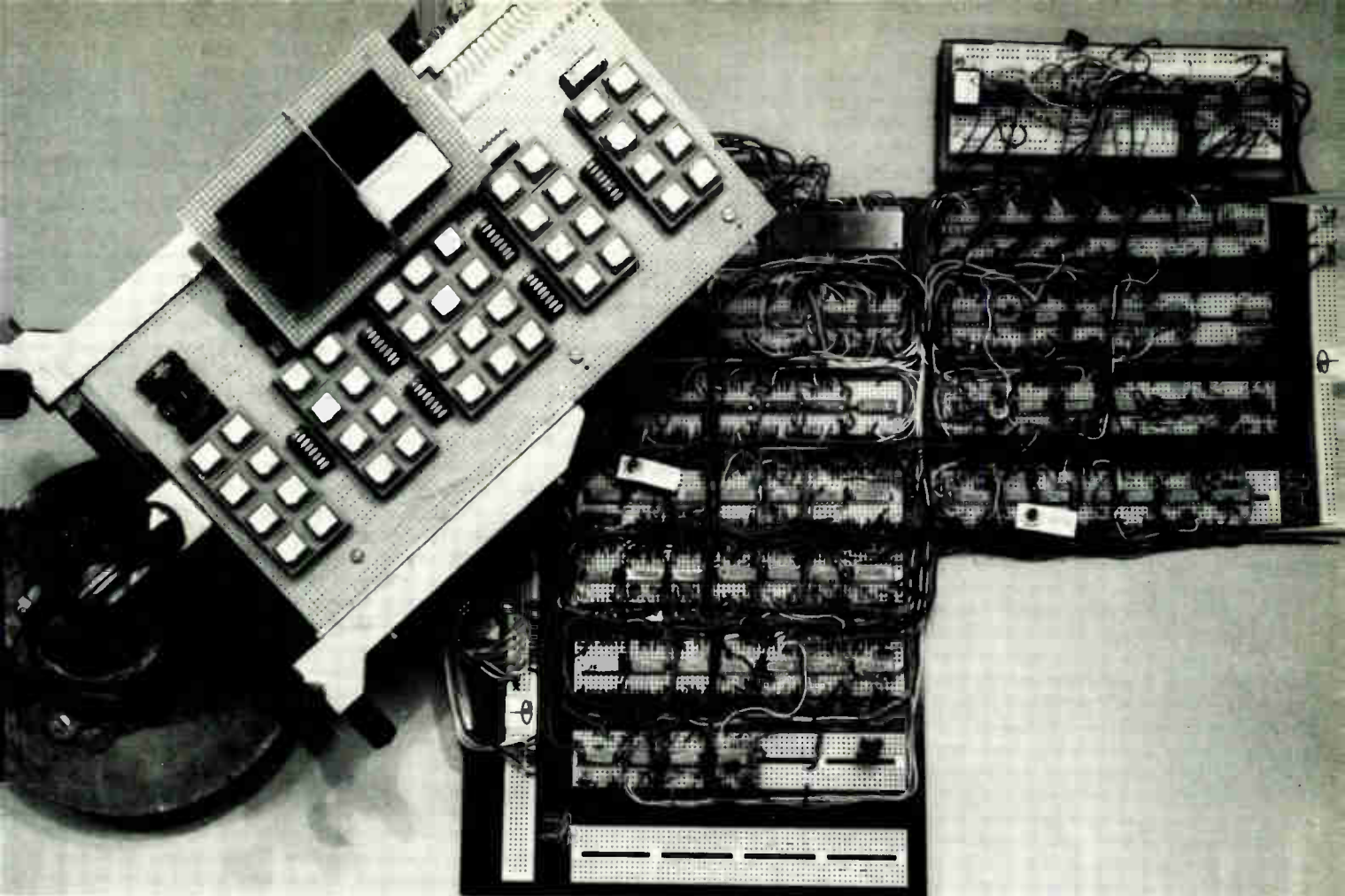
6. A mixture. This breadboard for a programable calculator from Picatinny Arsenal combines different systems. At left, a perforated board with the keyboard and display circuitry is mounted on a holding fixture. Other circuits and the wiring are on the two ranks of solderless breadboard sockets to the right. A stick-on copper wiring pattern serves as connector to the perforated board circuitry.
