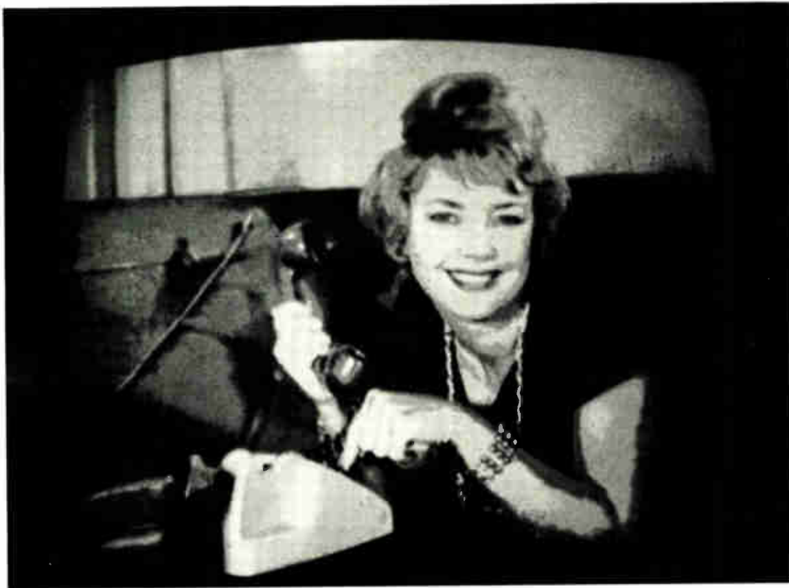
4. Clear picture. A composite NTSC video signal that has been encoded by 8-bit pulse-code modulation produces a good picture (top) on TV monitor. But same picture (bottom) with 3-bit encoding shows disturbing quantizing errors that would make it unsuitable for broadcasting. Therefore, it is necessary to find optimum bit-code rate without increasing bandwidth.
