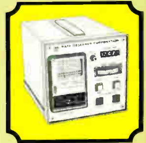
Data Research Transient Voltage Recorder
