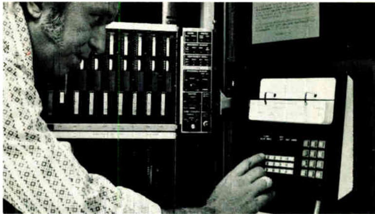
2. New tool. The control cabinet of the Dimension PBX contains a maintenance panel into which a "crafts-person," as he or she is called today, can key information necessary to change a customer's services. The panel also helps in diagnosing PBX troubles.
