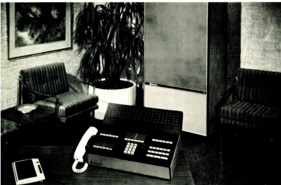
1. More than a switch. The first standard PBX in the Bell system, an 80-line, 15-trunk machine manufactured in 1904, was designed to serve as the standard switchboard. The newest PBX, introduced this year under the trademark Dimension, is an electronic, stored-program switching system that handles 400 lines and offers a myriad of features that can be changed simply by changing the software.
