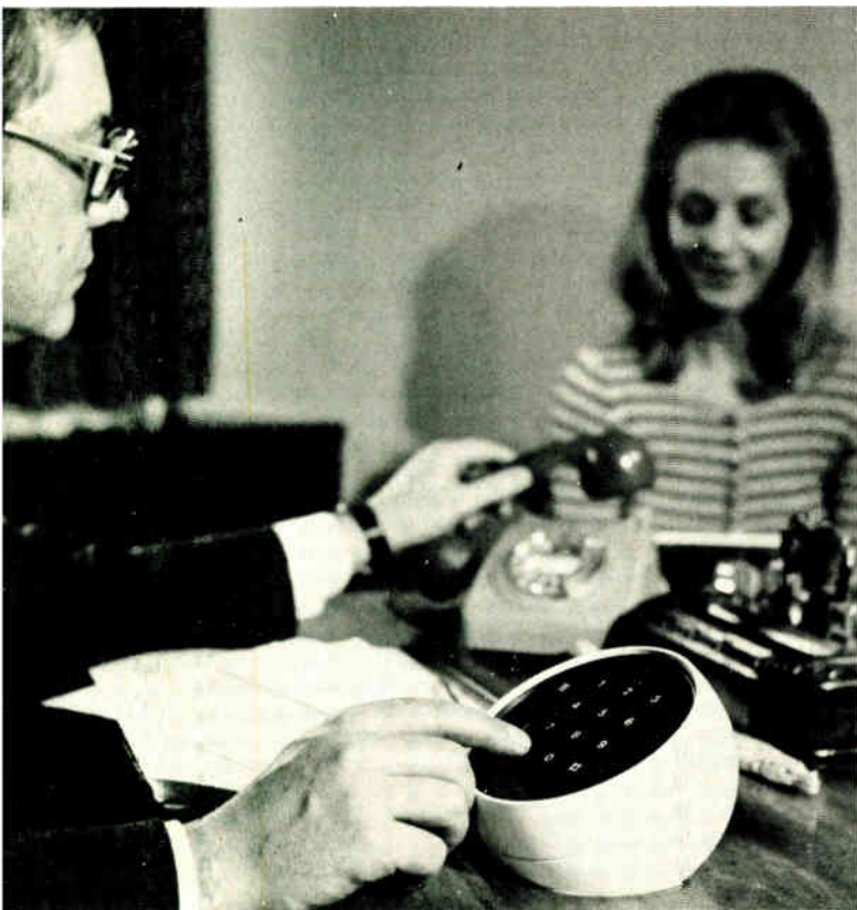
7. Programed push buttons. Pye TMC, England, has introduced its "SpheriCall" autodialer that adds push-button dialing to a standard rotary dial telephone and also stores 10 telephone numbers.
