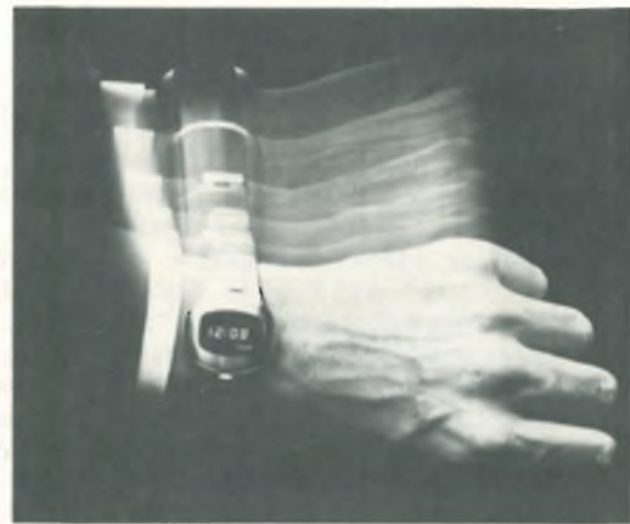
Fancy. Prototype watch/calculator from Optel shows time and has four-function calculator with liquid-crystal display. Pulsar's inertial switch turns on light-emitting-diode display with flick of wrist.
