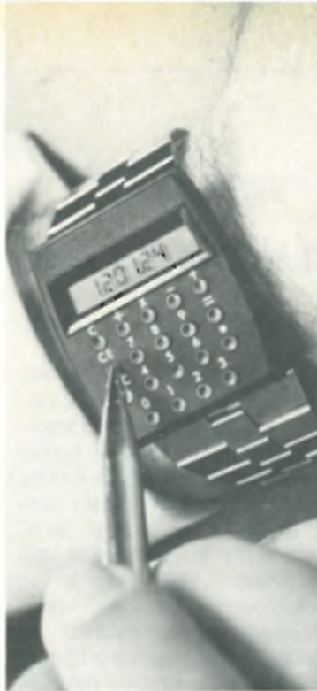
Fancy. Prototype watch/calculator from Optel shows time and has four-function calculator with liquid-crystal display. Pulsar's inertial switch turns on light-emitting-diode display with flick of wrist.
