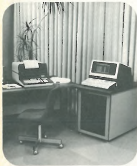
9882A subsystem (right) provides CRT and high speed data entry for 9830A calculator (left). Mass memory, below 9882A, has 4.8M bytes memory.
