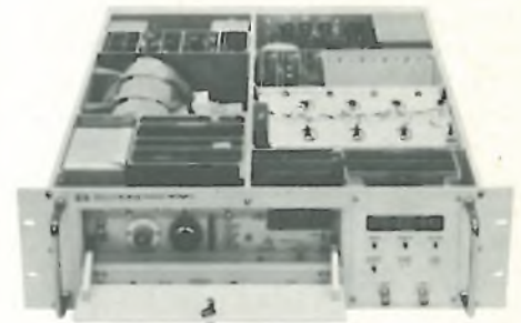
Remove the lid and you'll see the sturdy construction that enabled the 5062C Cesium Standard to pass the grueling 400-lb hammer blow test.
