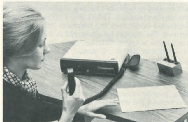
8. Disk dictation. The new IBM 6:5 Cartridge System for dictation employs magnetic disks, each disk holding six minutes of dictation, and 25 disks to a recording cartridge. Each recorder will hold two cartridges, thereby providing up to five hours of total capacity.
