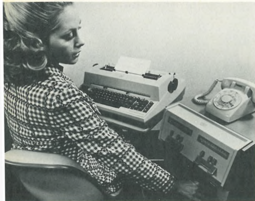
4. Typing by phone. Among the automated typewriters with communications capability is this Redactron unit. It performs information merging and editing using telephone-transmitted information. Advantage of system is ability to use data from various offices.
