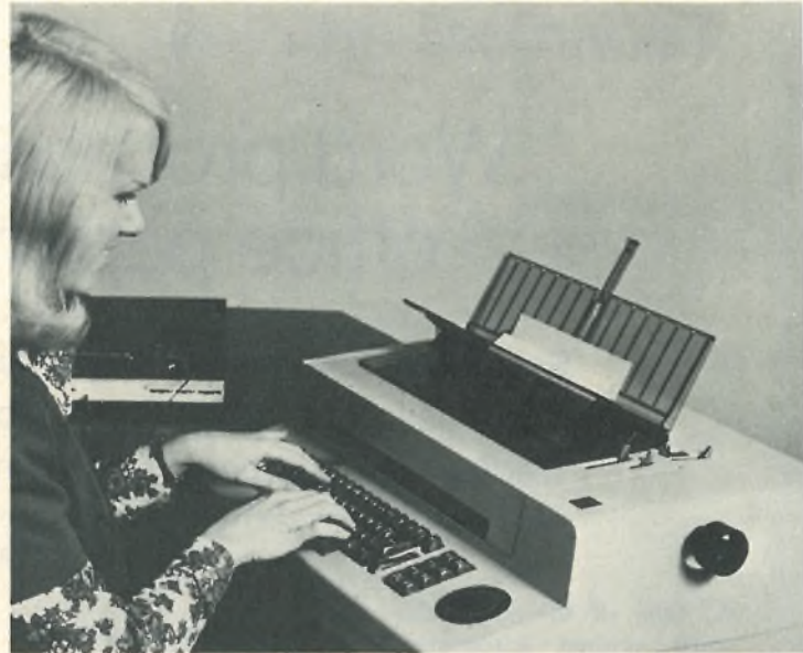
2. From number one. Two of the important word-processing machines from industry-leader IBM's extensive line are the Mag Card II (left), which has an 8,000-character memory, and the Memory Typewriter (above), a desk-top machine with 4-k memory.
