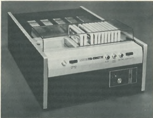
10. Talkative. A central dictation machine, the new Lanier Tel-Edisette, holds 12 standard audio cassettes that can be used in any of nine different recording modes covering one dictation per cassette, dictation shared with others, or telephone messages.
