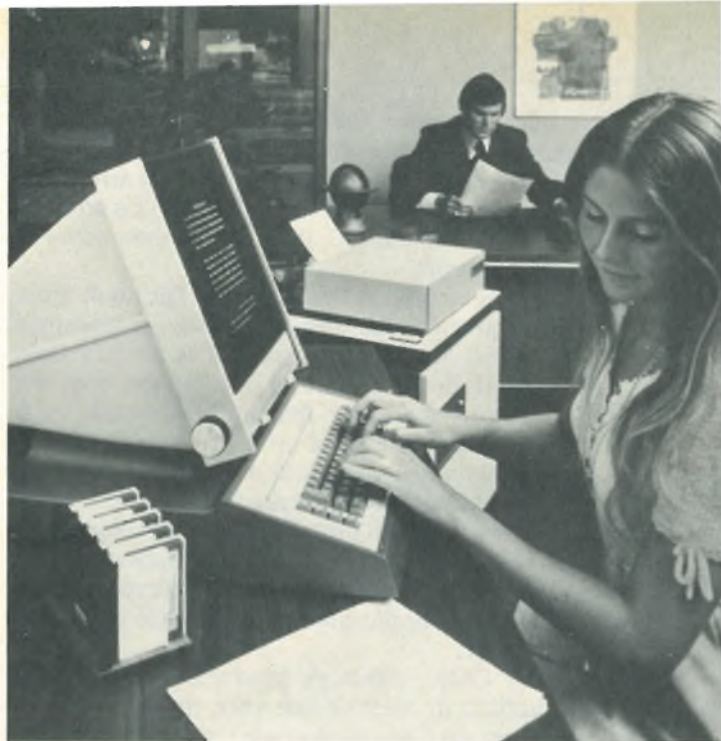
6. Video words. The Lexitron Videotype Text Processor Model 911 features a display that's oriented like a standard typewriter. When the operator types or turns the "roll-bar" handles on the side, the text "rolls up" from the bottom of the screen.
