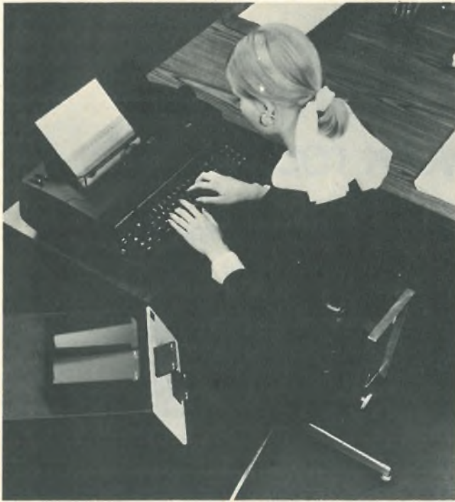
2. From number one. Two of the important word-processing machines from industry-leader IBM's extensive line are the Mag Card II (left), which has an 8,000-character memory, and the Memory Typewriter (above), a desk-top machine with 4-k memory.
