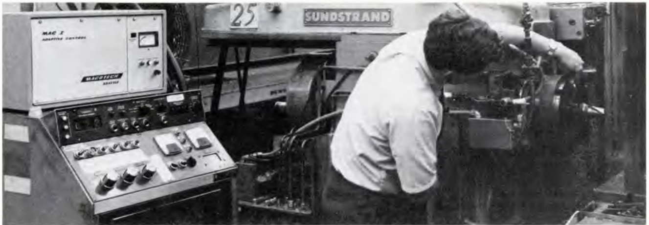
5. Deflection sensor. Sensor ring mounted on tool spindle detects spindle deflection, compares it with the maximum allowable value, and regulates machine speed accordingly. Adaptive control electronics are contained inside unit sitting on top of the NC controller.
