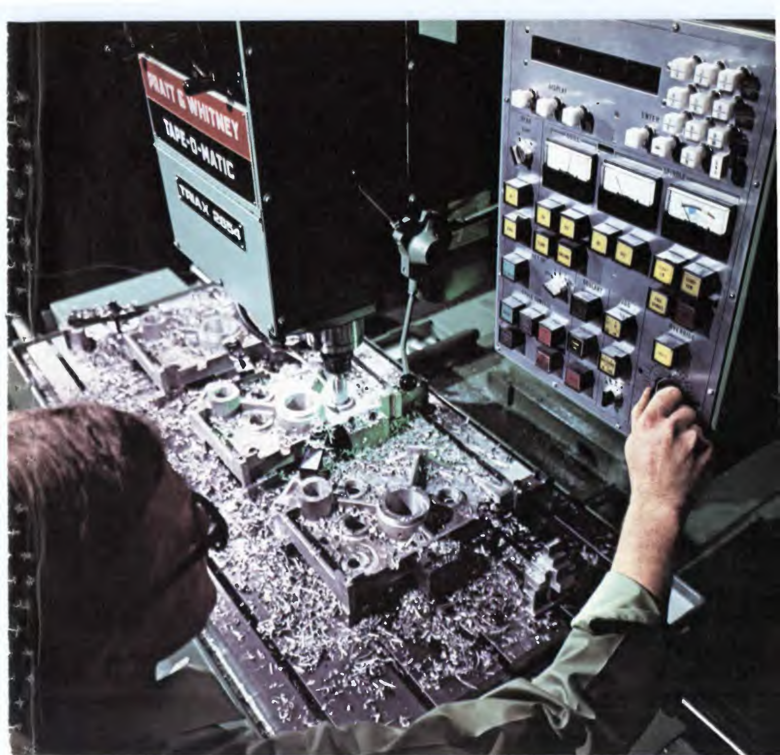
1. Numerical control. Operator adjusts jog speed on a Pratt & Whitney three-axis machining center, which is suitable for both small-lot and production jobs. Though inputs are normally entered on punched paper tape, data can be entered manually at the control panel.
