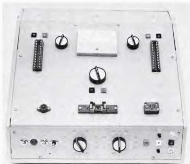
1. Analyzer. Most parameters of electronic components, and even functional modules and printed-circuit boards, can be checked with a sequential circuit analyzer. The two large sockets on the analyzer carry wired program cards for each device type. The device under test is connected via universal sockets on the sloping panel, and test conditions are set on the lower front panel.
