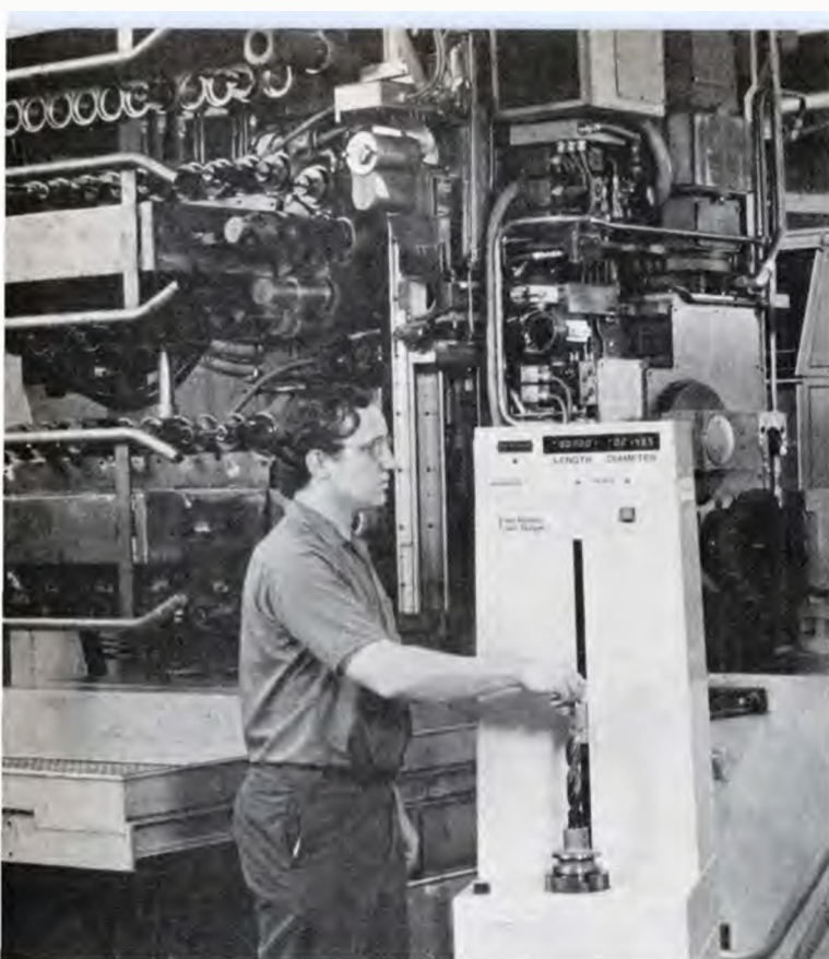
4. Automatic tool gaging. Operator electronically gages tool length for a 90-tool Cincinnati Milacron NC machining center. The length is registered on the LED display. After gaging, tool is inserted in whichever of the tool pockets, visible at the upper left, is appropriate.
