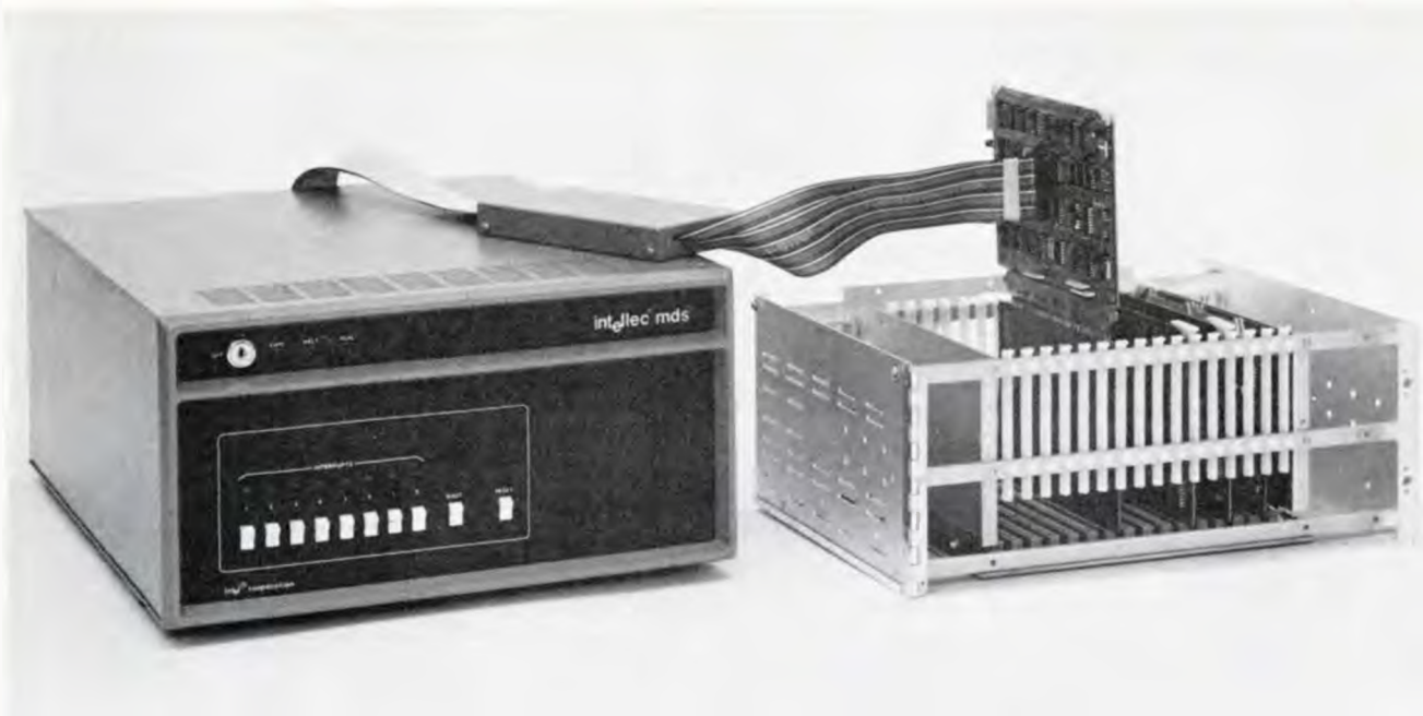
Uncut cord. An umbilical cable connects the Intellec MDS to the prototype equipment through a 40-pin dual-in line plug. The plug is inserted in the socket where either an 8080 microprocessor or a series 3000 bipolar microprogram-control unit will later be placed.
