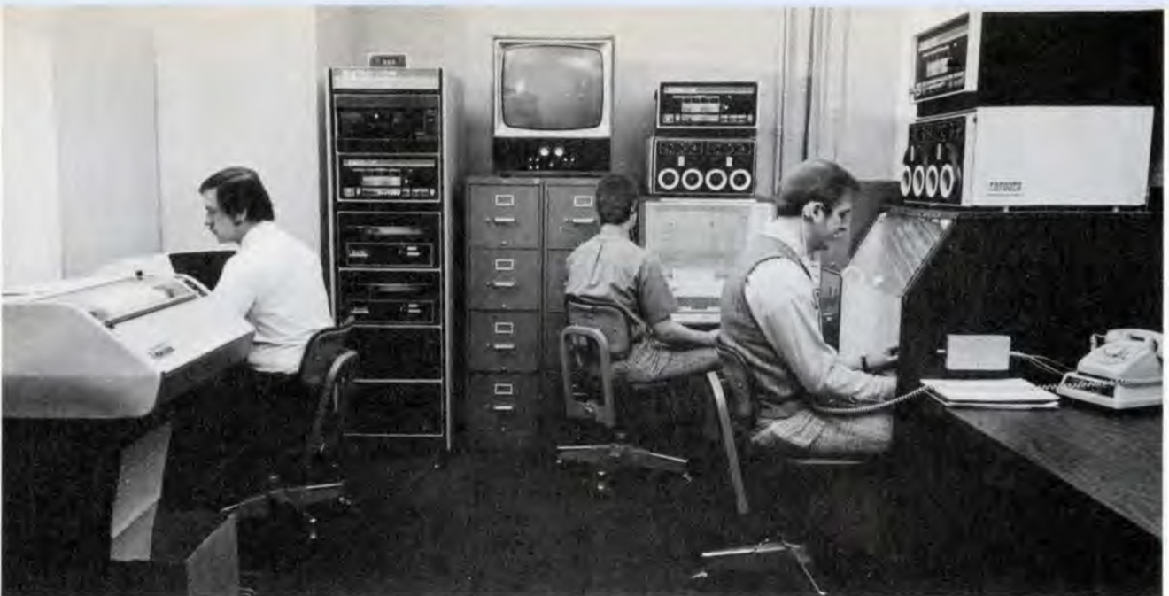
2. Diagnosing problems. When a Kearney & Trecker customer encounters a mechanical or electrical problem with his machine, he phones K & T's Diagnostic Center and connects his machine's CNC system to the Center's computer by means of a Data Phone modem. A diagnostic program is run on the machine, and the results are printed out and analyzed at the Center. Often the customer can do his own repairs.
