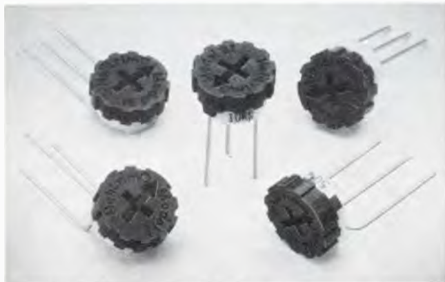
Pin money. By swaging instead of firing in the pins on these trimmers, Beckman Instruments makes manufacture easy to automate. Also, bending pins produces 12 different pin configurations.
