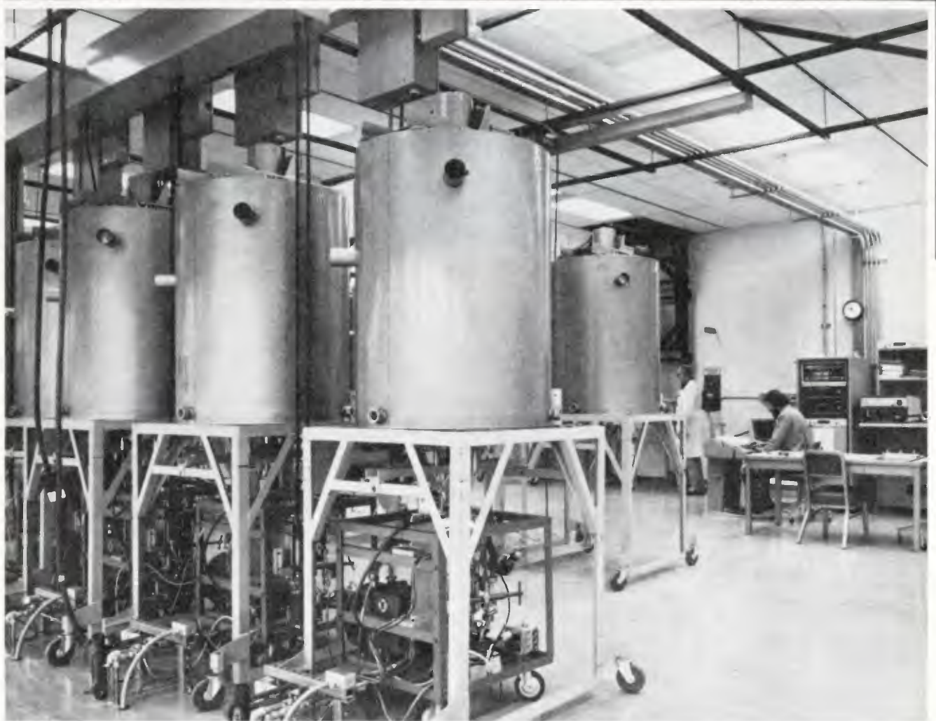
Elephant farm. Vacuum chambers at Tektronix are computer controlled for evacuation and sealing of cathode-ray tubes used in storage oscilloscopes. Units can be relocated, plugged into power sources, and run by one operator. Previous setups required two operators.
