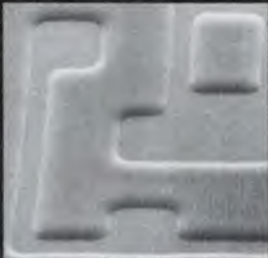
AZ-111 0.8 microns thick on silicon dioxide provides excellent edge acuity, etch resistance and line width control.
