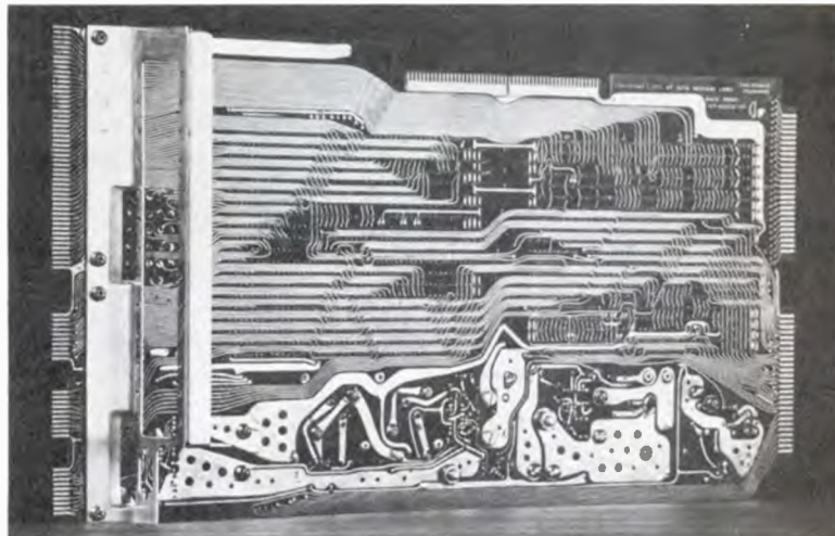
Engineered efficiency. When Data General put integrated power-supply circuitry into the backpanel on three Nova computers, back-panel wirewrapping was eliminated as well as much hand wiring.
