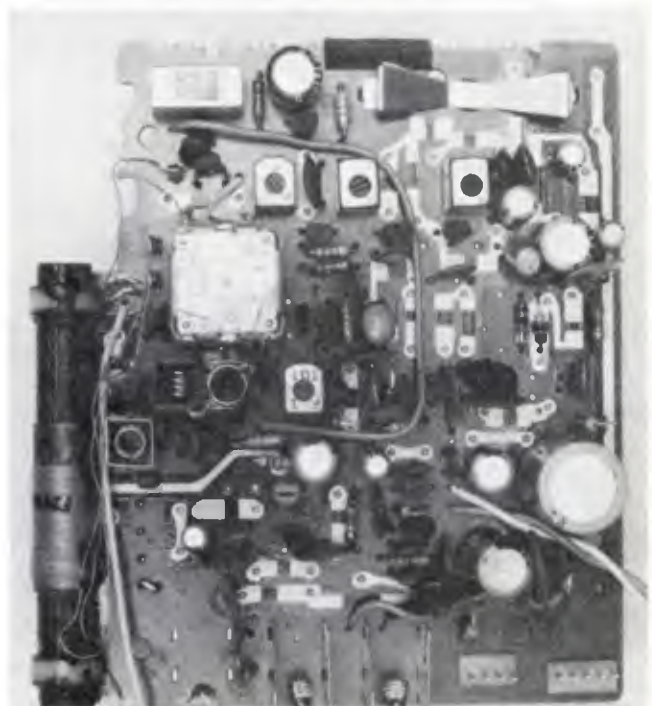
Tight fit. Radio circuit board built at Matsushita uses printed resistors (top photo) to ease space requirements where automatic insertion head must fit between densely placed components. Many of the parts on the completed board (bottom) are automatically inserted.
