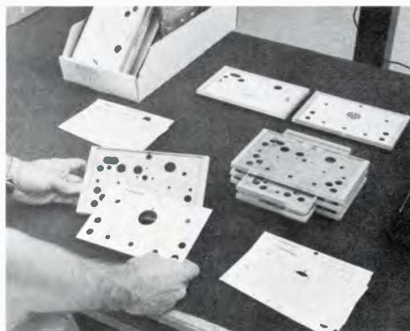
Simpler inventory. Wavetek uses the same pc boards (top) and front and rear panels (bottom) for different models.
