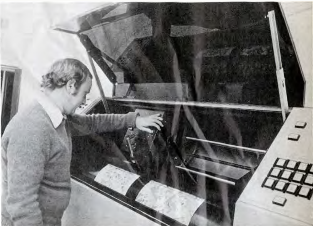
Printer. The optical scanner used in Sci-Tex Corp.'s design aid for the printing industry takes artist's pattern with as many as 12 different colors and converts it digital code. Design can then be manipulated via color crt.
