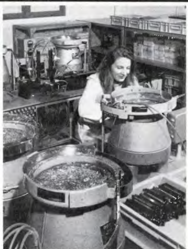
Contact. Machine at Socapex, a French connector manufacturer, inserts 50,000 contacts per day. One operator tends five machines.
