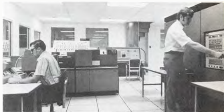
Productive storage. Automated purchasing and warehousing can make contributions to improving efficiency. At IBM Endicott's Materials Distribution Center (top), computer-controlled cranes patrol the shelves retrieving items ordered by an IBM 1800 (bottom).
