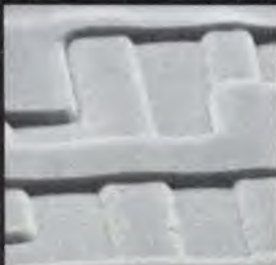
AZ-1350J on aluminum showing excellent step protection through the use of thick coatings.
