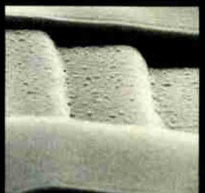
AZ-1350J allows "0" pinholing during etching.
