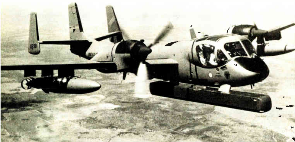
Data in a jiffy. Northrop Corp. transmission system sends data from side-looking radar, slung below Mohawk OV-1D fuselage, to the ground for processing while plane is in the air.
