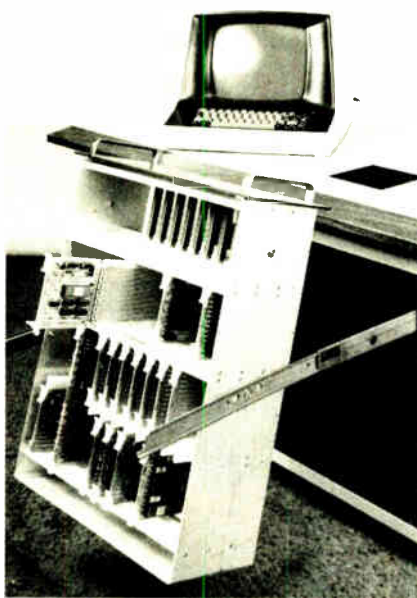
Test control. Drawer in system contains microprocessor and associated electronics.
