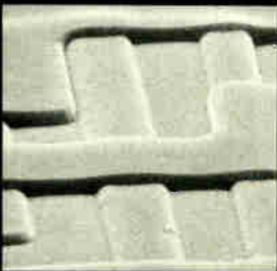
AZ-1350J on aluminum showing excellent step protection through the use of thick coatings.
