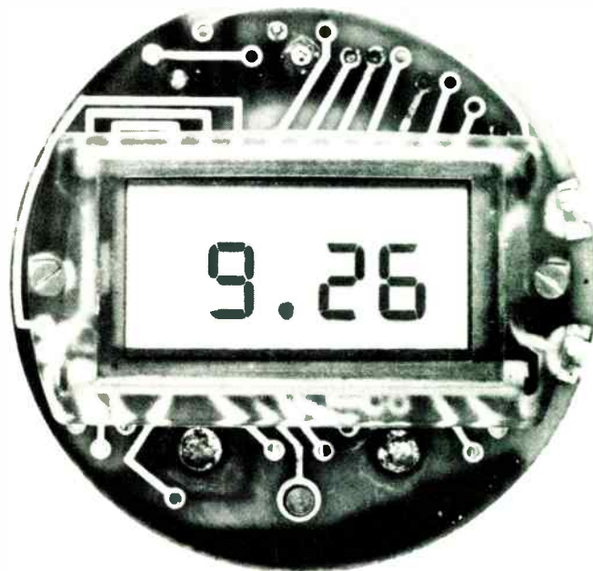
9. Swiss movement. The Nepro digital display module is one of the few Swiss electronic watches. It's got U.S.-made C-MOS ICs and a Swiss-made field effect LCD, lighted for visibility in the dark.
