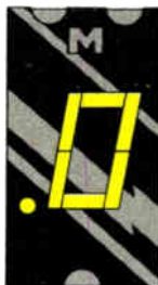
MAN 82 Common Anode; Left Hand Decimal
