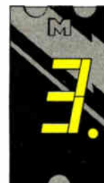
MAN 84 Common Cathode; Right Hand Decimal
