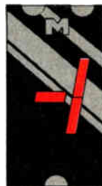
MAN 73 Common Anode; Overflow ( \pm 1 )
