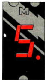
MAN 71 Common Anode; Right Hand Decimal
