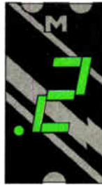
MAN 52 Common Anode; Left Hand Decimal
