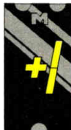
MAN 83 Common Anode; Overflow ( \pm 1 )
