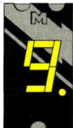
MAN 81 Common Anode; Right Hand Decimal
