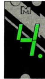
MAN 54 Common Cathode; Right Hand Decimal
