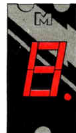
MAN 74 Common Cathode; Right Hand Decimal
