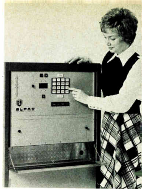
Detector. Microprocessor-based spectrometer makes drug tests automatically.
