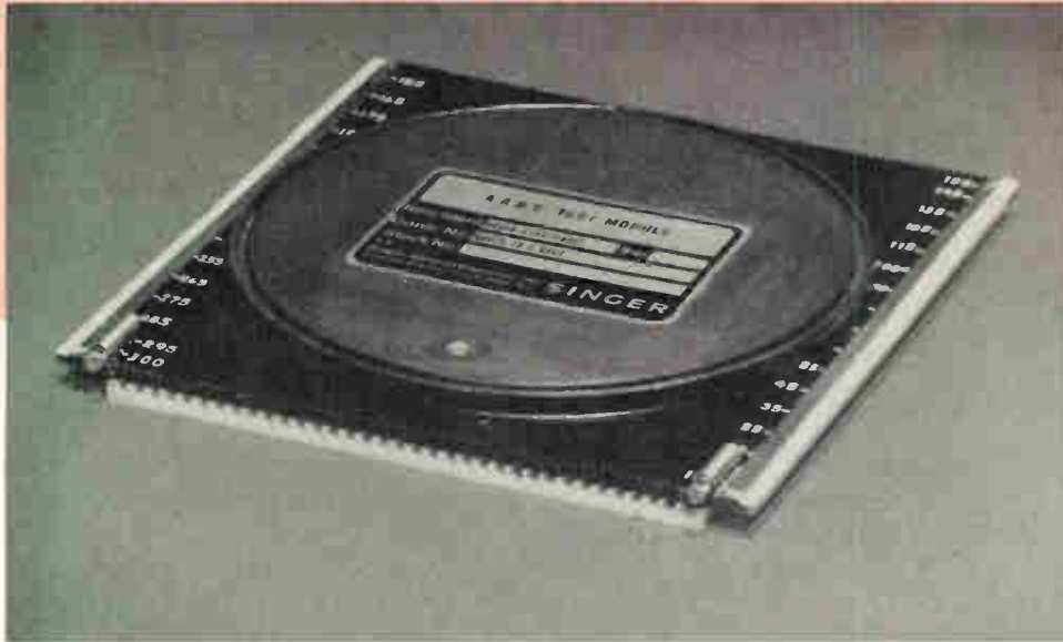
5. A cool water. Efficient thermal package houses a 3-inch LSI wafer (a). Component parts (b) include an alumina or beryllia heat exchanger that fastens directly to the base ceramic, optimizing cooling. Substituting more costly beryllia enhances thermal conductivity by a factor of 12.
