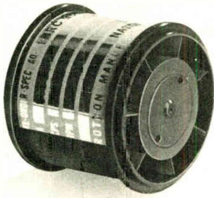
4. Breezes to order. This fan weighs only an ounce, fits in a 1-inch cube, and is well suited for microelectronic applications. Rotron, the manufacturer, rates life expectancy in excess of 20,000 hours. Device delivers up to 8 cubic feet per minute.
