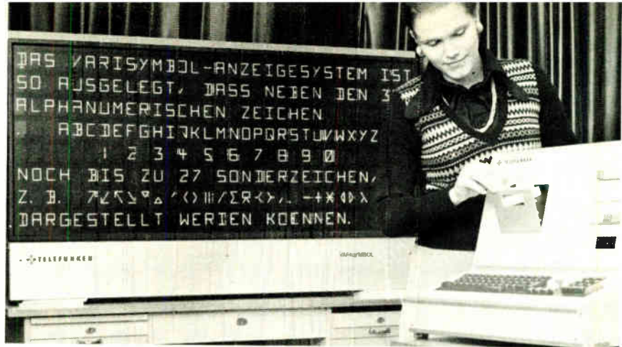
All aglow. AEG-Telefunken's gas-discharge display allows 27 special symbols in addition to 36 alphanumerics. Decimal point and position indicator are available, too.
