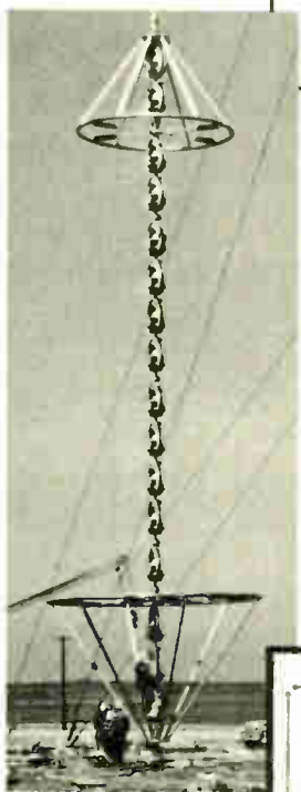
Large structural-guy insulator assembly with grading rings
