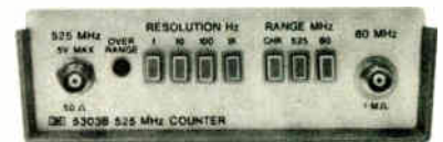
5303B — 525 MHz Counter Module: DC to 525 MHz range, burst or CW frequency. 50 \Omega or 1 M \Omega input. Automatic gain control. Fuse protected front end. Optional high stability time base (FCC Type-Approved). $800.
