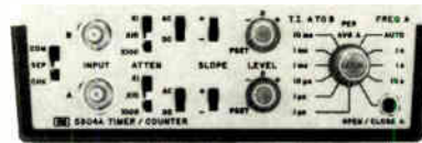
5304A — 10 MHz Timer/Counter Module: DC to 10 MHz range. 100 nsec. time interval accuracy. Unique "Time Interval Holdoff" ignores input ringing or contact bounce. Two DC coupled amplifiers with attenuators, slope, polarity and gain control. $325.
