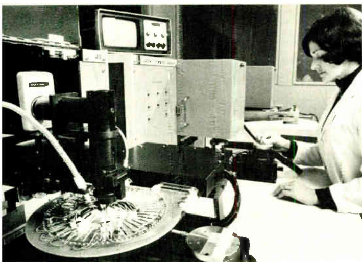
Trimming them up. Laser trimming systems have become standard tools for tailoring resistance values to specified tolerances. These systems—at Garrett Manufacturing Ltd., Rexdale, Ont. (left) and Beckman's facility in Fullerton, Calif (right)—are completely computer controlled for automatic trimming of thick- and thin-film circuits in both substrate and packaged form. Most systems in use include an automatic probing unit that determines whether the individual resistors printed in the substrate require laser trimming.
