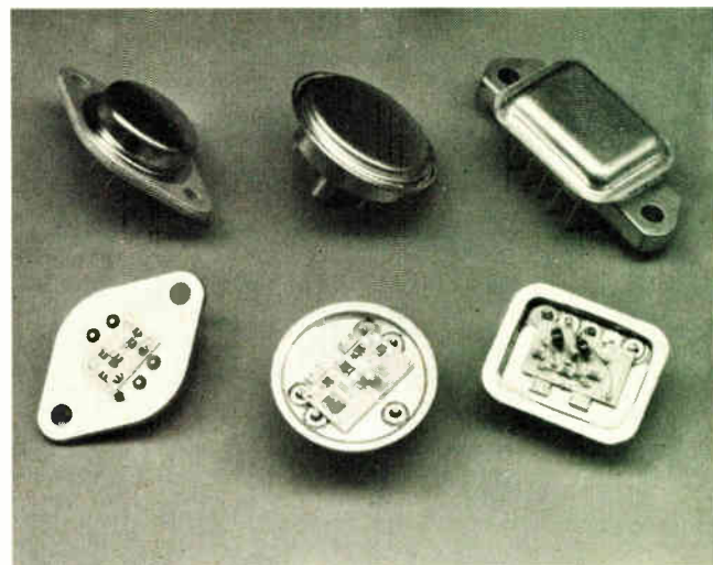
The high and the mighty. High power and high frequency are areas illustrating how thick-film technology can be tailored to design goals. The 10-A device (left), by International Rectifier, on a BeO substrate comes in a standard TO-3 package. Replacing two SCRs and three diodes, this small unit can be compared to IR's older 25-A and 42.5-A hybrids also shown. Thick-film hybrids are also pushing up the performance of uhf and vhf modules. These standard modules (right), with active devices on separate substrates, are by Motorola.
