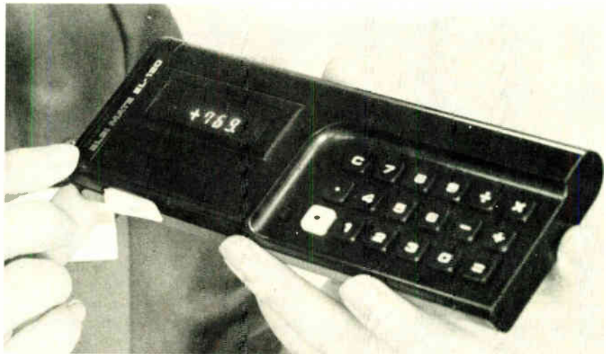
Low cost. Although Sharp's new calculator has only three-digit display, its circuitry handles a 12-digit number and gives serial display.
