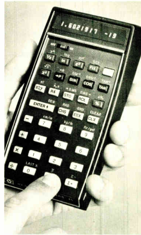
Packs a wallop. This is a 47-operation machine with nine addressable registers.
