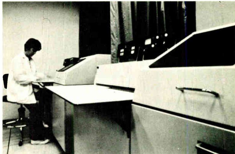
Trimming them up. Laser trimming systems have become standard tools for tailoring resistance values to specified tolerances. These systems—at Garrett Manufacturing Ltd., Rexdale, Ont. (left) and Beckman's facility in Fullerton, Calif (right)—are completely computer controlled for automatic trimming of thick- and thin-film circuits in both substrate and packaged form. Most systems in use include an automatic probing unit that determines whether the individual resistors printed in the substrate require laser trimming.
