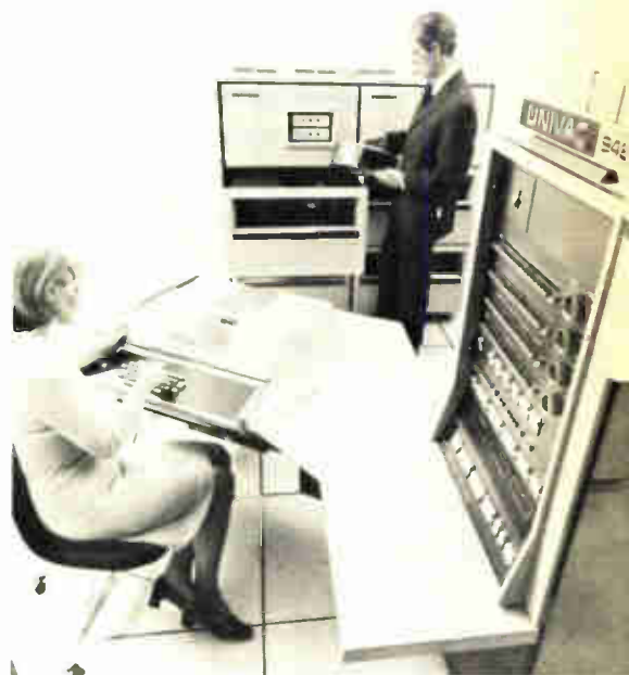
No plated wire here. Univac's 9480 has a semiconductor main memory; it is a medium-scale system using 1103s.
