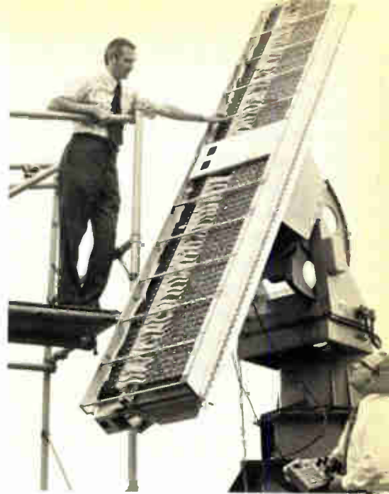
MLS entry. The Bendix-Bell-Lockheed scanning-beam antenna has 81 elements and operates in C band.
