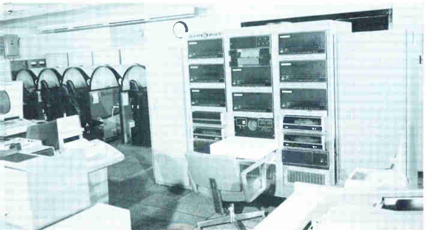
4. Portent. Prized by Data General Corp. is this network of eight Nova minicomputers, part of a General Electric Co. simulation system for training Navy pilots. The minicomputer network is an increasingly important way to get high performance at low cost.
