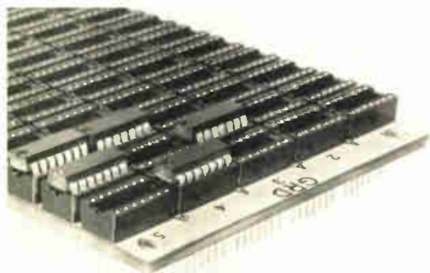
1. Pin-in-board. For dual in-line-device mounting, low-profile board (0.060 inch maximum above panel) may be wired on the back for varying circuit applications. Board is priced between 85 cents and $1.50 per device, based on two devices per square inch.
