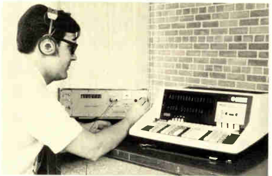
Finding his place. Engineer tunes in simplified Transit satellite signal receiver (Transim) at Johns Hopkins Applied Physics Lab. At right is the standard electronic desk calculator.
