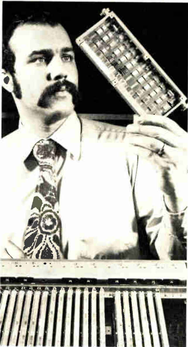
4. One-sided. In RCA's computers, components are soldered to single-sided eight-layer boards plugged to a backplane. One or two rows of cards make up one subunit—a central processor, an I/O processor, or a memory—that mounts in a liquid-cooled frame.
