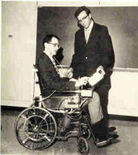
Voice control. Electric wheelchair is controlled by hums picked up by the throat microphone.
