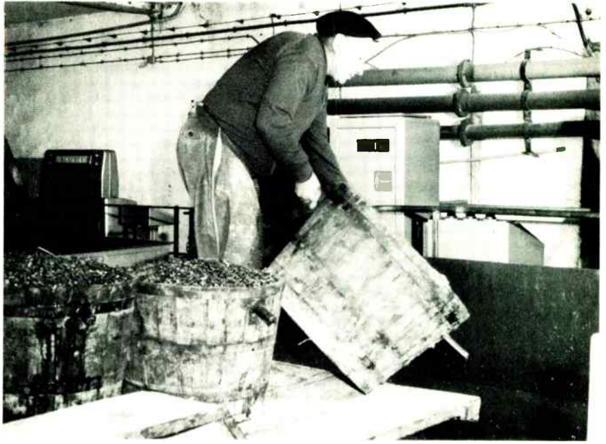
Hands off. Automatic refractometer equipment in French winery replaces manual methods of determining grape's sugar content and potential alcohol content.
